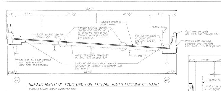
Note 1. Additional full depth removal may required at locations of existing floor drains, as directed by Engineer. Anticipated removal and replacement quantities included in pay items for "Concrete Removal" and "Concrete Superstructure".
