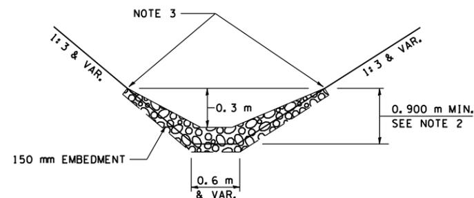
STONE DUMPED RIPRAP DITCH CHECK
