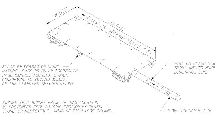
REMOVE SILT WHEN BAG IS HALF FULL OR MORE OFTEN IF RECOMMENDED BY THE MANUFACTURER. DISPOSE OF SILT BY TRANSPORTING THE FILLED BAG TO DISPOSAL AREA. SLIT THE BAG, BLEND SILT INTO EXISTING TOPOGRAGHY, SEED AND MULCH
