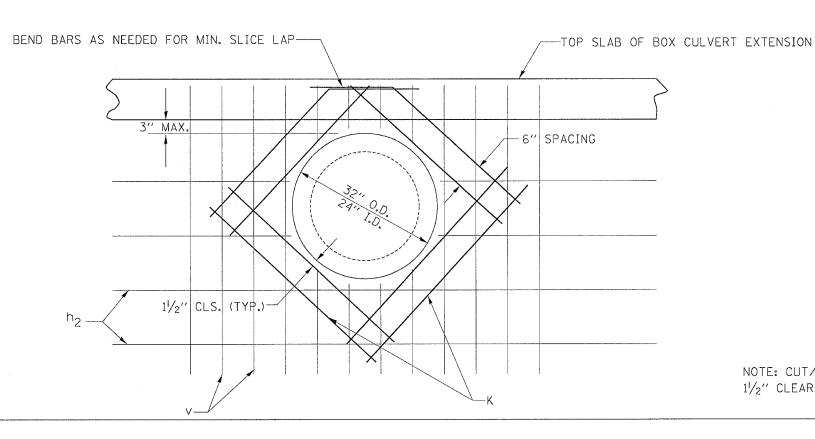
NOTE: CUT/TRIM  $h_2$  AND v BARS AS NEEDED TO PROVIDE  $1^1/2^{\prime\prime}$  CLEARANCE AROUND STORM SEWER PIPE.
