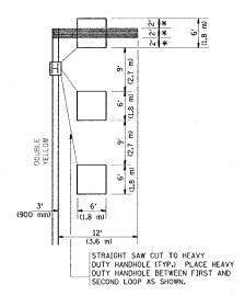
PLAN SHEET FOR DETECTOR LOOP REPLACEMENT
