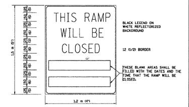
THESE SIGNS ARE REQUIRED ON BOTH SIDES OF THE RAMP, 4 MINIMUM OF I WEEK IN ADVANCE OF THE CLOSURE.
