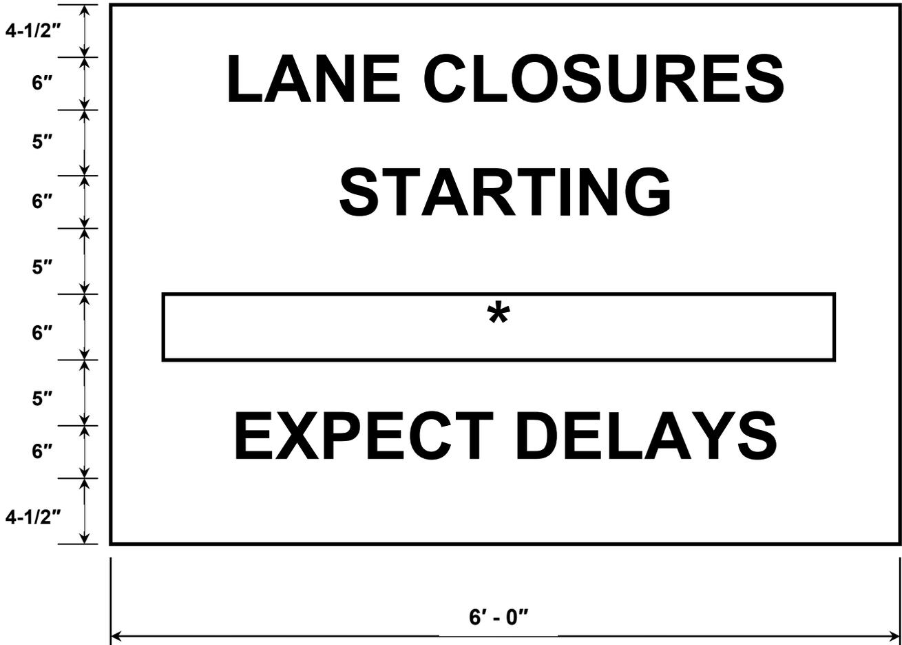
**\* CONTRACTOR SHALL PROVIDE DATE FOR START OF LANE CLOSURE AND SHALL ERECT SIGNS A MINIMUM OF ONE (1) WEEK IN ADVANCE OF THE START OF THE WORK.**
