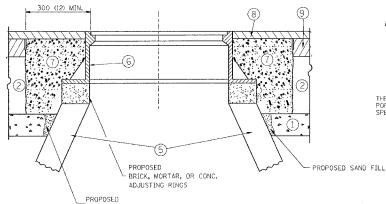
EXISTING BROKEN FRAMES AND LIDS SHALL BE REMOVED AND DISPOSED OF BY THE CONTRACTOR AND SHALL BE REPLACED AS DIRECTED BY THE REGINEER. REPLACEMENT FRAMES AND LIDS WILL BE PAID FOR IN ACCORDANCE WITH ARTICLE 109,04 OF THE STANDARD SPECIFICATIONS UNLESS A SEPARATE PAY ITEM HAS BEEN PROVIDED.
