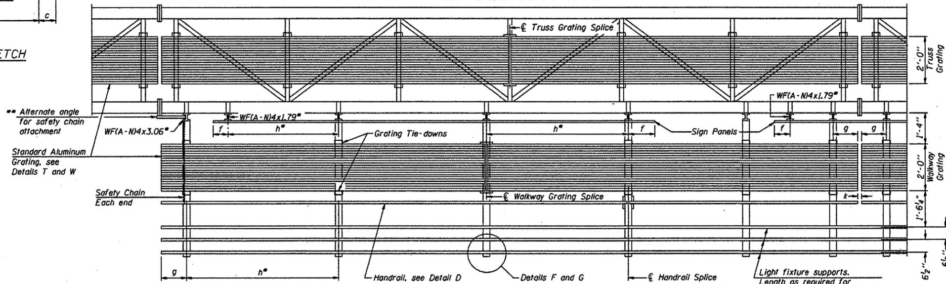
Walkway and Truss Grating width dimensions are nominal and may vary  $\pm 1/2$ " based on available standard widths.
