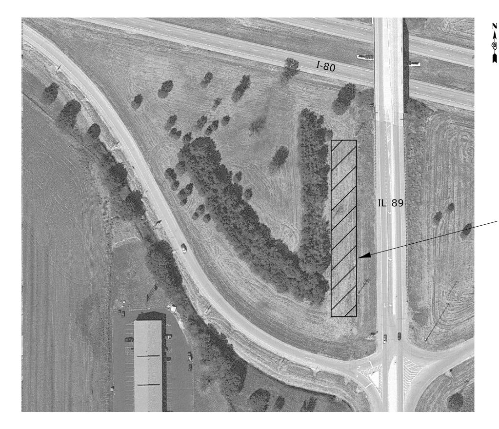
PLACE THE EXCAVATED MATERIAL FROM THE MOW STRIP IN APPROXIMATELY A 400' x 50' AREA. THE AREA SHALL BE SEEDED AND MULCHED AS DESCRIBED IN THE PLANS AND SPECIAL PROVISIONS.
