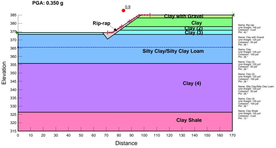
IL 13 over Crab Orchard Creek Overflow (SN 039-0019) East Abutment (Boring 2-S) w/ Abutment Pile Seismic Analysis
