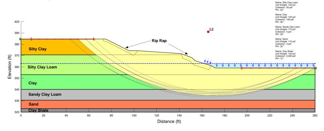
IL 13 over Crab Orchard Creek (SN 039-0061) West Slopes (Boring 1-S) with Piles Seismic Analysis PGA: 0.350 g
