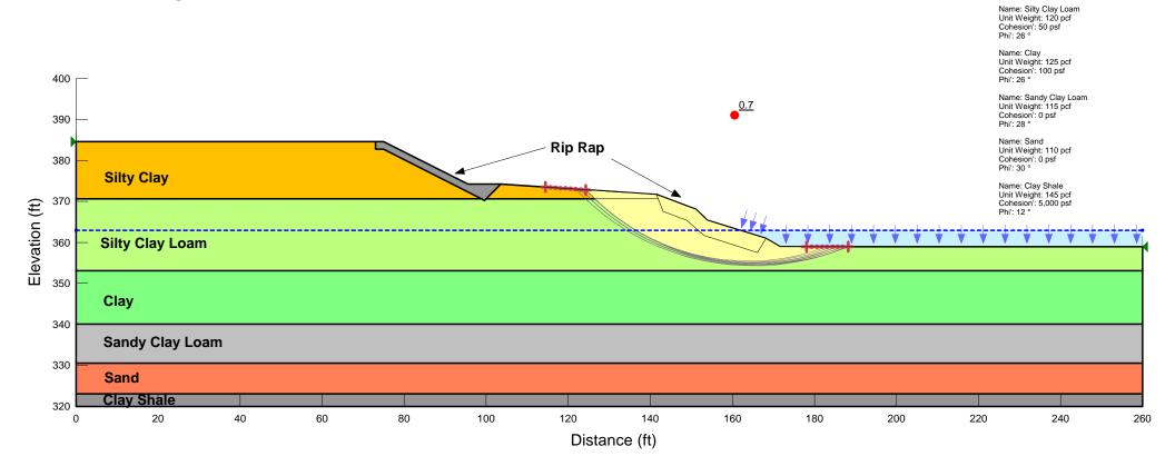
IL 13 over Crab Orchard Creek (SN 039-0061) West Bottom Slope (Boring 1-S) with Pile Seismic Analysis PGA: 0.350 g
