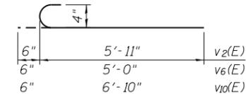
**BARS v<sub>2</sub>(E), v<sub>6</sub>(E) and v<sub>10</sub>(E)**
