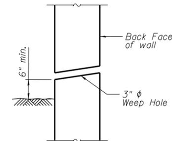
**WEEP HOLE DRAIN DETAIL**
