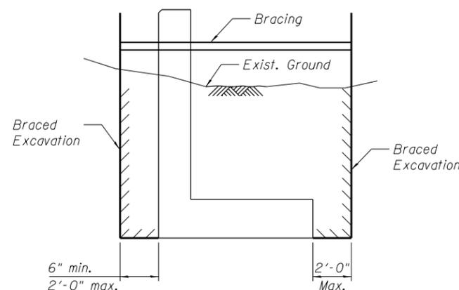
**BRACED EXCAVATION DETAIL**
