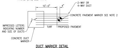
SURFACE COURSE DUCT MARKER -BASE COURSE #10 PULL WIRE COIL A MINIMUM OF 3' AT DUCT ENDS. INSTALL APPROVED PLUGS IN END OF DUCTS NOT USED.
