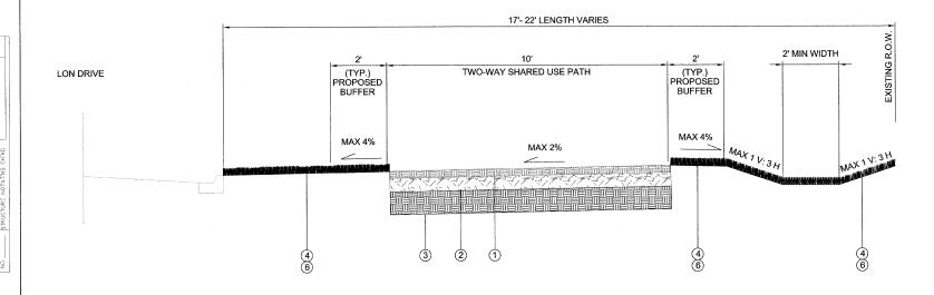
TYPICAL CROSS SECTION FOR TWO-WAY SHARED USE PATH STA 210+77.10 TO 212+83.00
