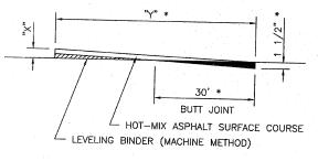
"X" = PROPOSED PAVEMENT THICKNESS
