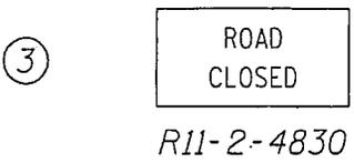
*Mount on Type III Barricades as shown on Std. 701901 Detail for "ROAD CLOSED TO ALL TRAFFIC". Each Type III Barricade shall have two Type A Flashing Lights.*
