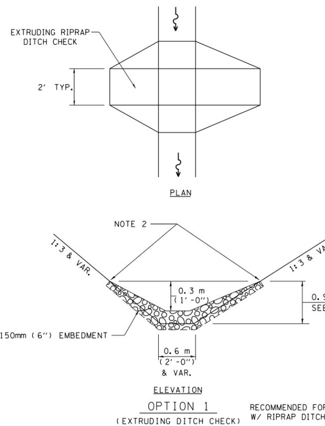
**STONE DUMPED RIPRAP DITCH CHECK**
