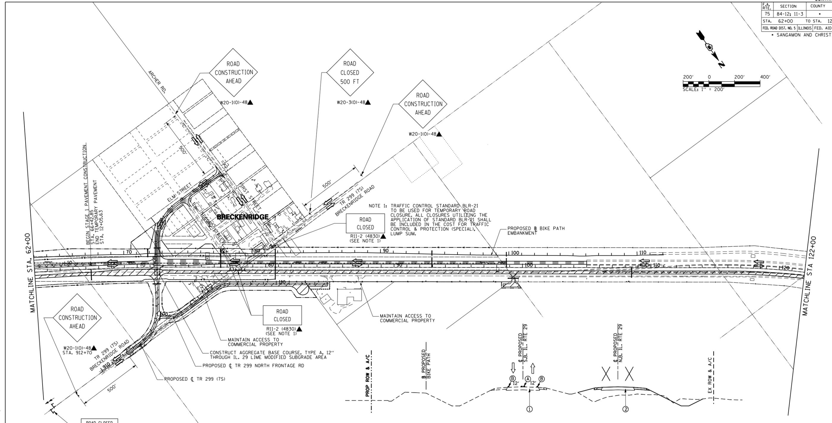
NOTE 1: TRAFFIC CONTROL STANDARD BLR-21 TO BE USED FOR TEMPORARY ROAD CLOSURE. ALL CLOSURES UTILIZING THE APPLICATION OF STANDARD BLR-21 SHALL BE INCLUDED IN THE COST FOR TRAFFIC CONTROL & PROTECTION (SPECIAL), LUMP SUM.
