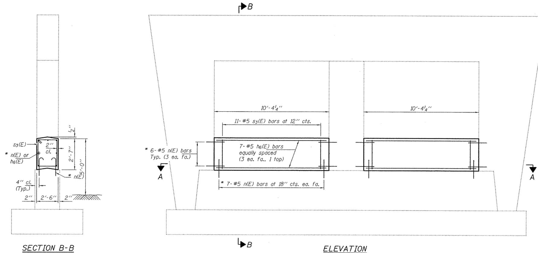
\* Epoxy grout n(E) bars in 9" min. holes according to Article 584 of the Standard Specifications.
