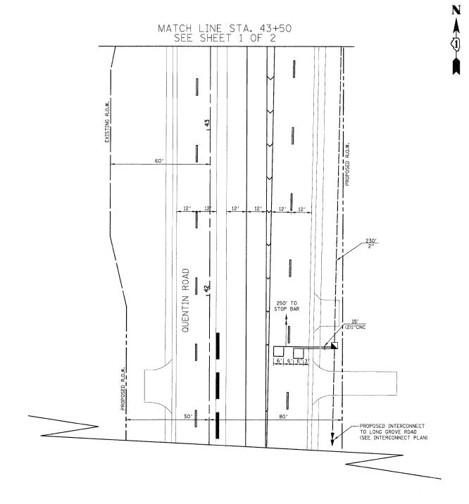
NOTE: THE TRAFFIC SIGNAL CONTROLLER EQUIPMENT FOR THIS PROJECT SHALL BE "ECONOLITE" AND NTCIP COMPLIANT TO MATCH THE EXISTING ADJACENT SYSTEM.
