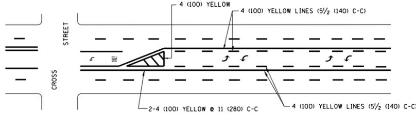
A MINIMUM OF TWO PAIRS OF TURN ARROWS SHALL BE USED, WHITE IN COLOR. ADDITIONAL PAIRS SHALL BE PLACED AT 200' (60 m) TO 300' (90 m) INTERVALS.
