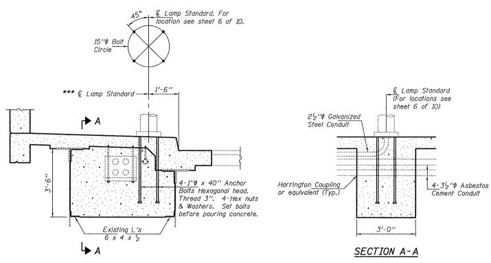
SECTION THRU SIDEWALK AT LIGHT STANDARD
