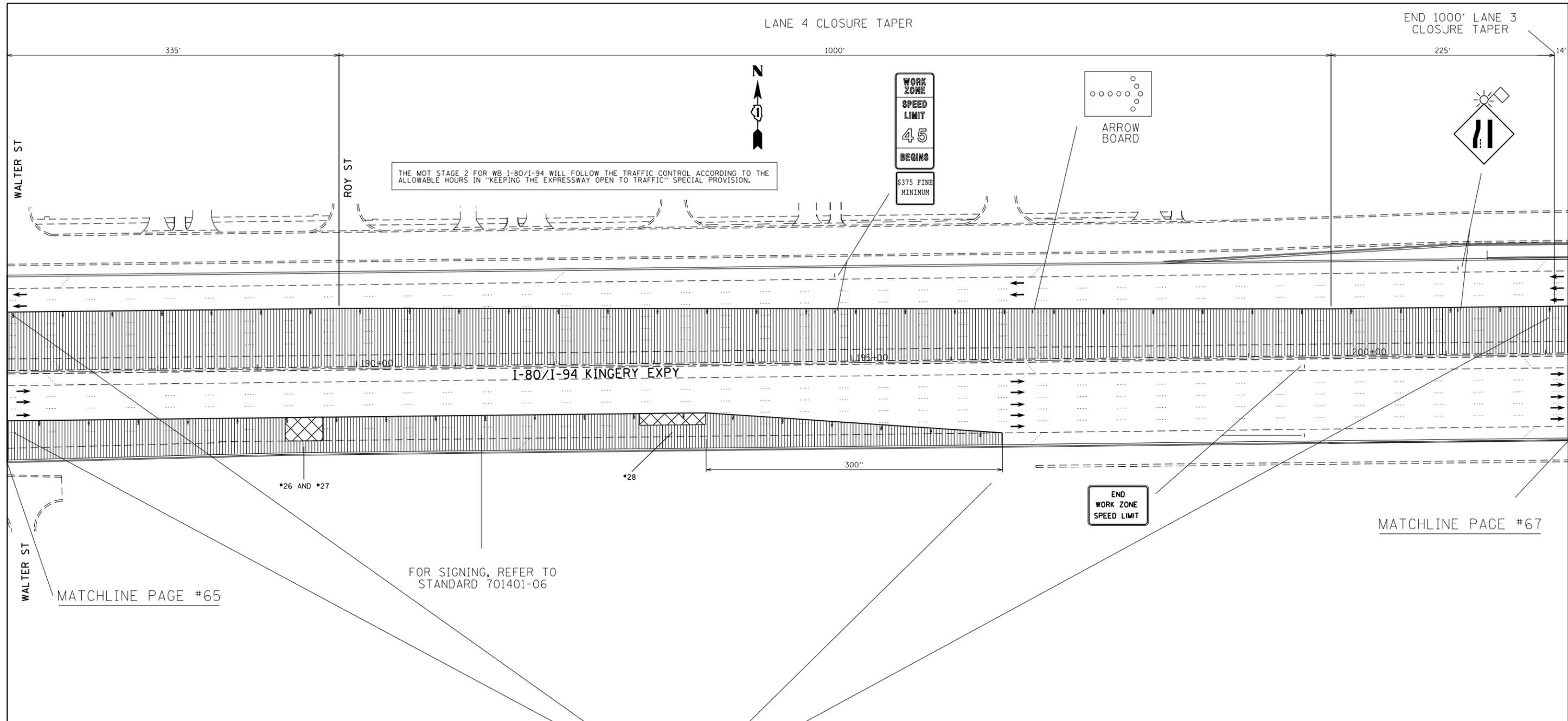
THE MOT STAGE 2 FOR WB I-80/I-94 WILL FOLLOW THE TRAFFIC CONTROL ACCORDING TO THE ALLOWABLE HOURS IN "KEEPING THE EXPRESSWAY OPEN TO TRAFFIC" SPECIAL PROVISION.
