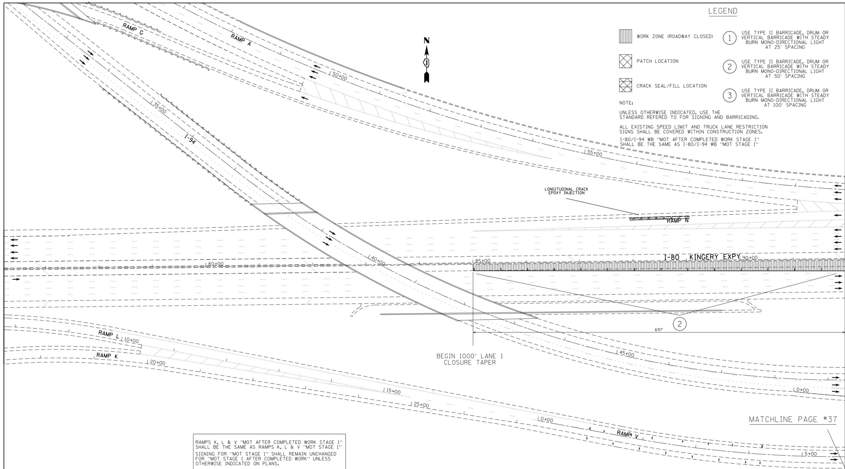
RAMPS K, L & V "MOT AFTER COMPLETED WORK STAGE 1" SHALL BE THE SAME AS RAMPS K, L & V "MOT STAGE 1" SIGNING FOR "MOT STAGE 1" SHALL REMAIN UNCHANGED FOR "MOT STAGE 1 AFTER COMPLETED WORK" UNLESS OTHERWISE INDICATED ON PLANS.
