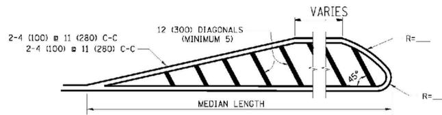
FOR MEDIAN LENGTHS WHERE DIAGONAL SPACING CANNOT BE ATTAINED, USE 5 (FIVE) EQUALLY SPACED DIAGONAL LINES.
