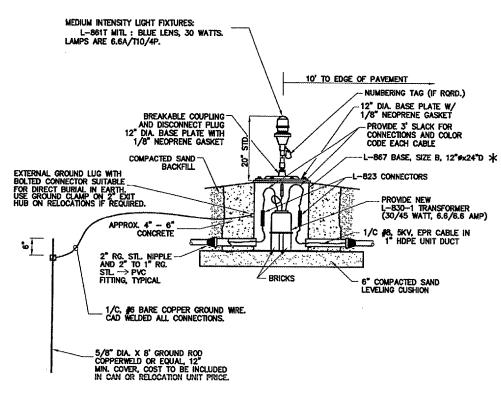
L-861T EDGE LIGHT INSTALLATION / RELOCATION DETAILS
