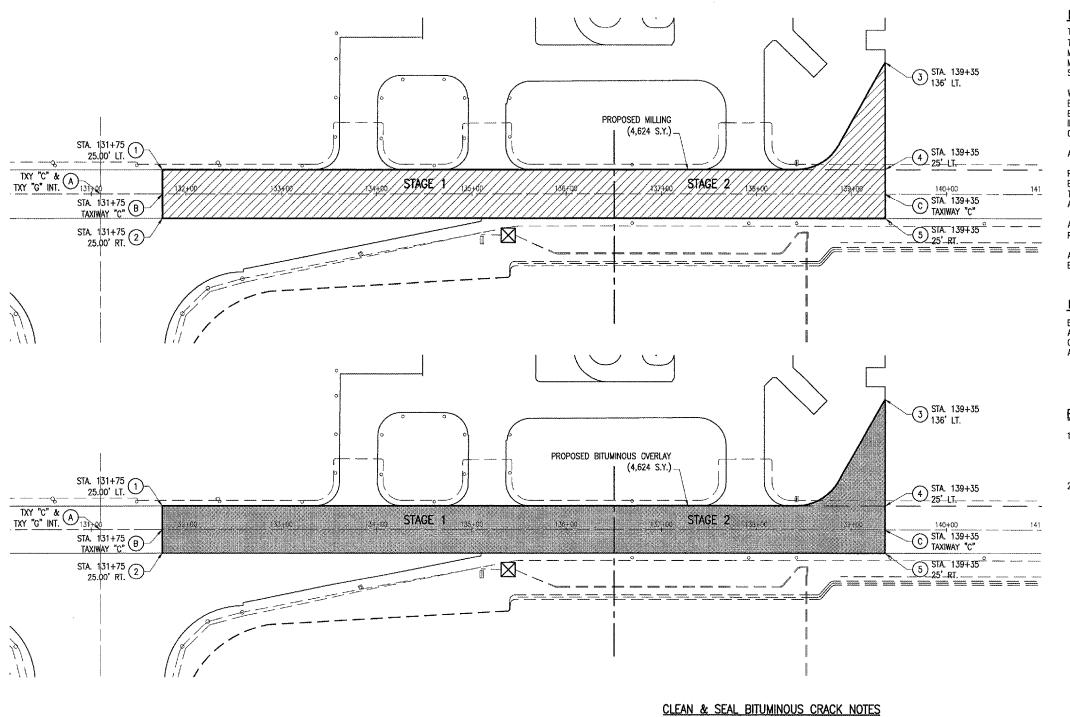
FOLLOWING A VISUAL SURVEY OF THE EXISTING PAVEMENT SURFACE, A PROPOSED PLAN QUANTITY OF 500 LINEAR FEET OF CRACK CLEANING AND SEALING WAS ESTABLISHED. THE EXACT AMOUNT OF CRACKS TO BE CLEANED AND SEALED WILL BE THE NUMBER OF LINEAR FEET OF CRACKS MARKED BY THE RESIDENT ENGINEER.
