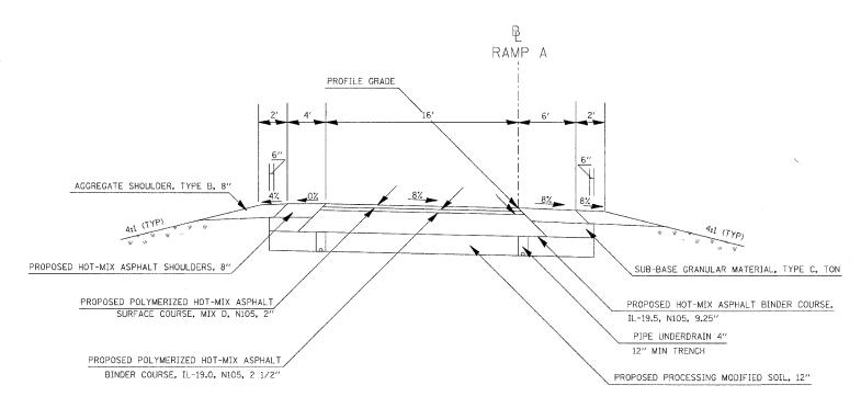
ATTAIN SUPERELEVATION STA 312+18.35 TO STA 314+78.35
