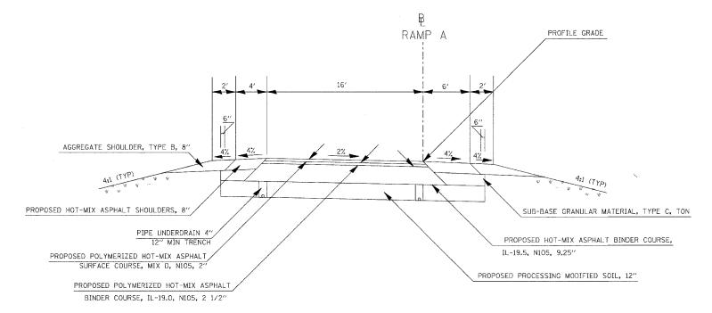
ATTAIN SUPERELEVATION STA 312+18.35 TO STA 314+78.35
