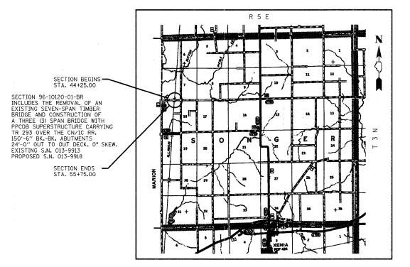
LOCATION: NEAR THE NW CORNER, NE 1/4, NW 1/4, SECTION 18, T3N, R5E, 3RD P.M. NET LENGTH OF SECTION 96-10120-01-BR: 1150.00 FT = 0.218 MI
