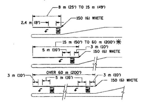
\* TURN LANES IN EXCESS OF 120 m (400') IN LENGTH MAY HAVE AN ADDITIONAL SET OF ARROW - "ONLY" INSTALLED MIDWAY BETWEEN THE OTHER TWO SETS OF ARROW - "ONLY".
