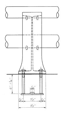
NOTE: Aluminum railing support post are to be removed, cleaned and reinstalled during construction. New bolts, bearing pads, and post support anchor assemblies are to be provided. (4 Locations)
