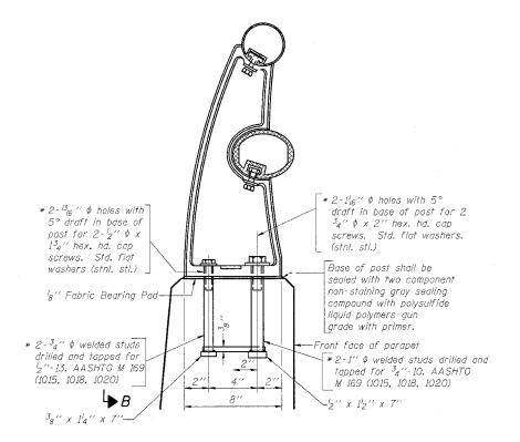
\* In lieu of the cast-in-place anchor device shown, the Contractor has the option of drilling and epoxy grouting stainless steel anchor rods of the same diameter and grade as the specified cap screws. Embedment shall be according to the manufacturer's specifications.
