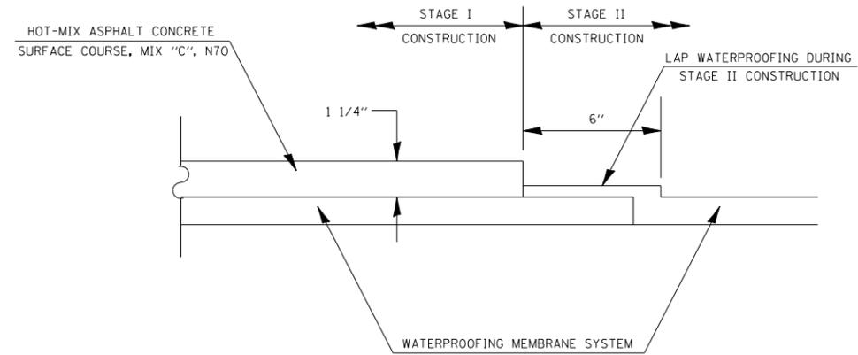
**WATERPROOFING TREATMENT AT STAGE CONSTRUCTION**
