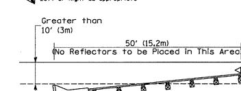
Begin reflectors at 10' (3m) point but no closer than 50' (15.2m) to terminal -Edge of shoulder
