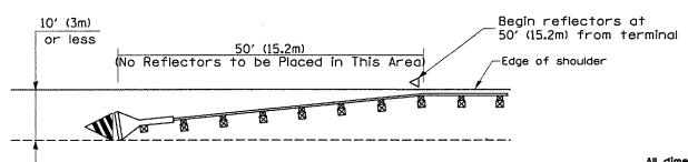
Traffic Barrier Terminal Type 1(Specia) [Terminal 10' (3m) or less from edge of shoulder] All dimensions are in inches (millimeters) unless otherwise noted.
