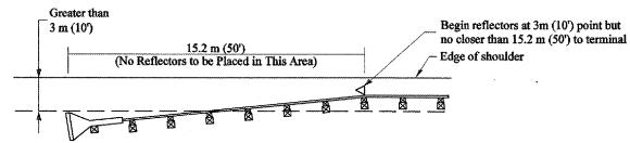
NOTE: Omit terminal marker when terminal over 3m (10') from edge of paved shoulder or break point of unpaved shoulder.
