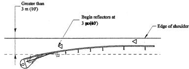
NOTE: Omit terminal marker when terminal over 3 m (10°) from edge of paved shoulder or break point of unpaved shoulder, or when terminal buried in backslope.
