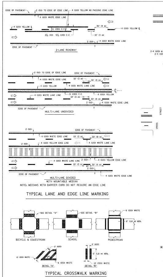
2-4 (100) YELLOW @ 11 (280) C-C-4' (1.2 m) DITSIDE TO NO DIAGONALS OUTSIDE OF LINES - 2-4 (100) YELLOW @ 11 (280) C-C 4' (1.2 m) WIDE MEDIANS ONLY 12 (300) DIAGONALS 2-4 (100) @ 11 (280) C-C 2-4 (100) @ 11 (280) C-C-
