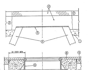
BRICK, MORTAR, OR CONC. ADJUSTING RINGS
