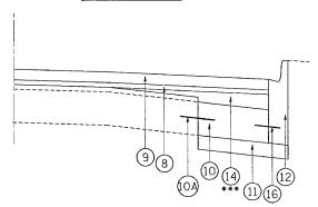
\*\*\* USE LEVELING BINDER FOR CROSS SLOPE CORRECTION
