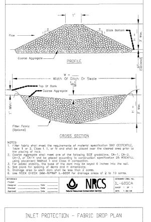
ROCK CHECK DAM - COARSE AGGREGATE
