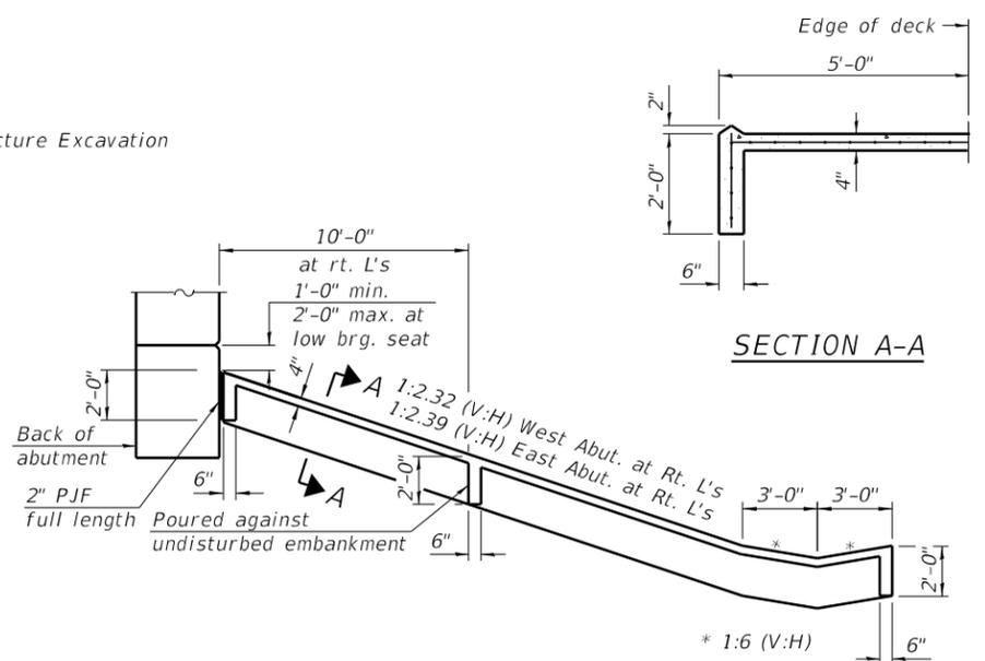
SECTION THRU CONCRETE SLOPEWALL
