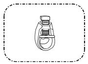
¾" (20mm) HEAVY-DUTY GROUND ROD CLAMP (BURNDY TYPE GRC OR APPROVED EQUAL)
