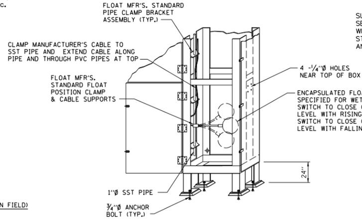
**ENLARGED FLOAT DETAIL IN STILLING WELL ENCLOSURES**
