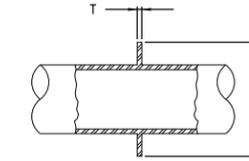
**DUCTILE IRON WALL PIPE COLLAR DIMENSIONS DETAIL**
