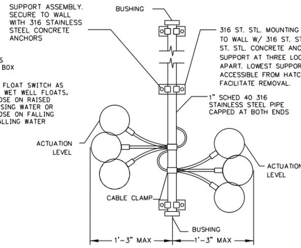
**ENLARGED FLOAT DETAIL STILLING WELL REMOVED**
