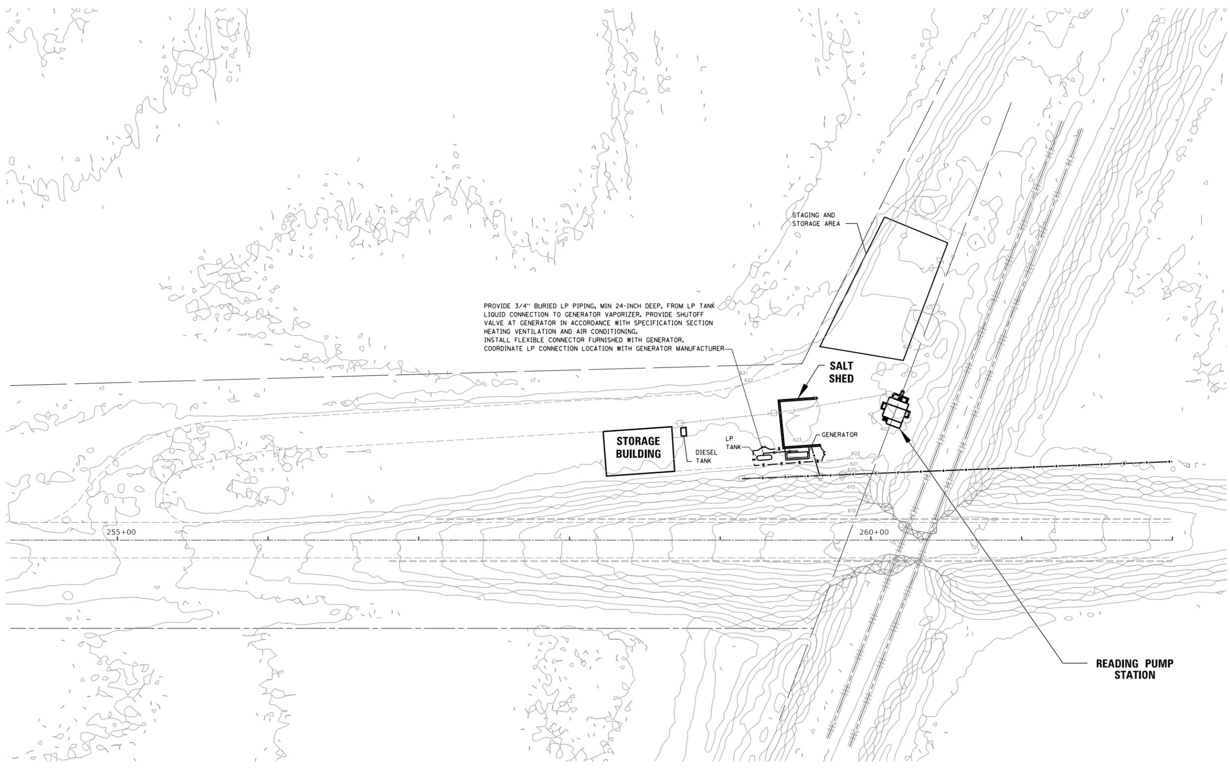
PROVIDE 3/4" BURIED LP PIPING, MIN 24-INCH DEEP, FROM LP TANK LIQUID CONNECTION TO GENERATOR VAPORIZER. PROVIDE SHUTOFF VALVE AT GENERATOR IN ACCORDANCE WITH SPECIFICATION SECTION HEATING VENTILATION AND AIR CONDITIONING. INSTALL FLEXIBLE CONNECTOR FURNISHED WITH GENERATOR. COORDINATE LP CONNECTION LOCATION WITH GENERATOR MANUFACTURER.
