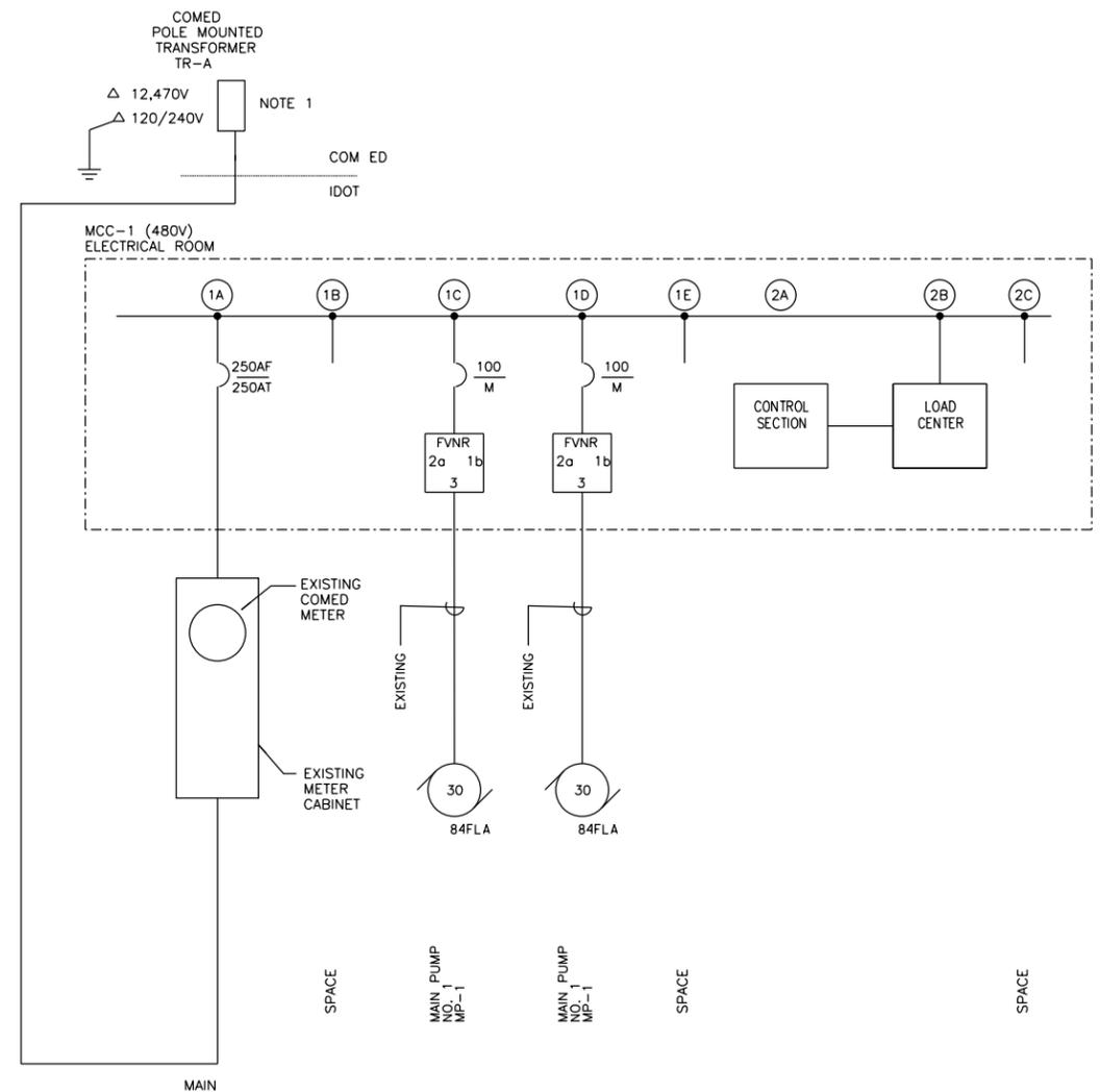
**OVERALL ONE-LINE DIAGRAM - REMOVAL
