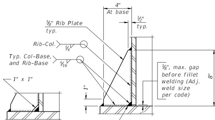
\*\* Alternate detail if welding col. to base plate first, then snip inside corner of ribs. Terminate weld on rib 1/4" from snip.
