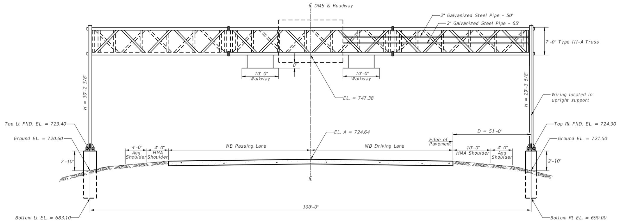
SIGN TRUSS MOUNTING DETAIL
