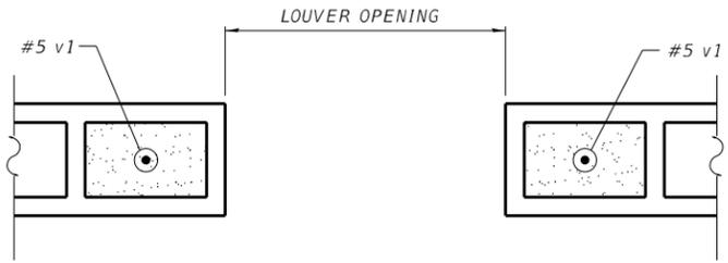
MASONRY WALL LOUVER OPENING DETAIL
