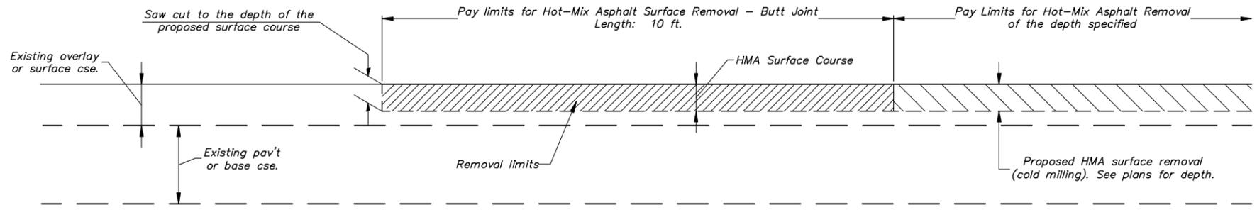
**CASE 2: BUTT JOINT & SURFACE REMOVAL w/ RESURFACING**
