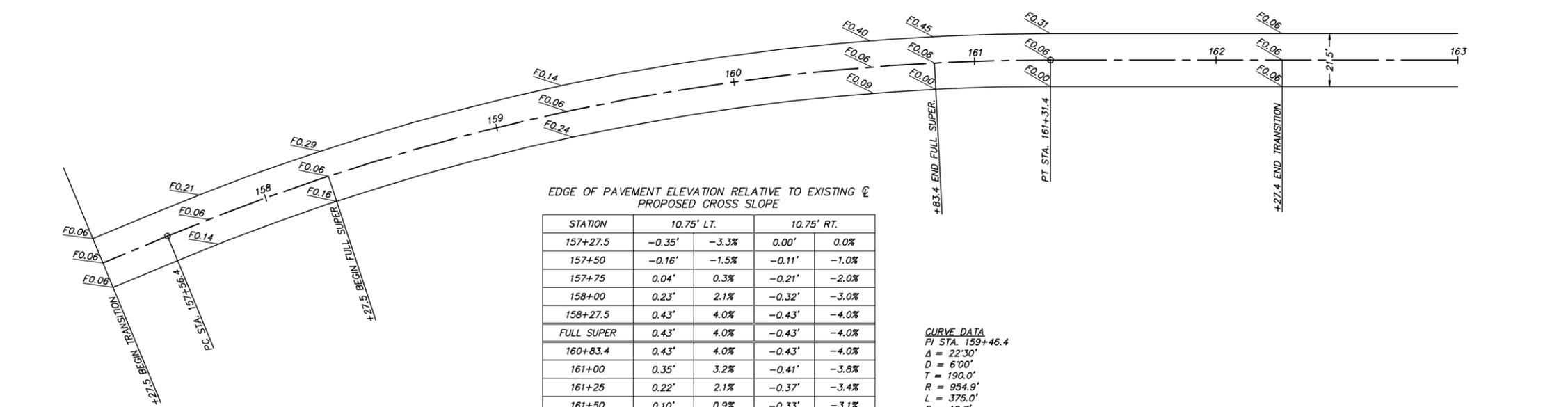
F = THICKNESS OF LEVELING BINDER REQUIRED TO OBTAIN DESIRED CROSS SLOPE AT THAT STATION INCLUDING FINAL LIFT.
