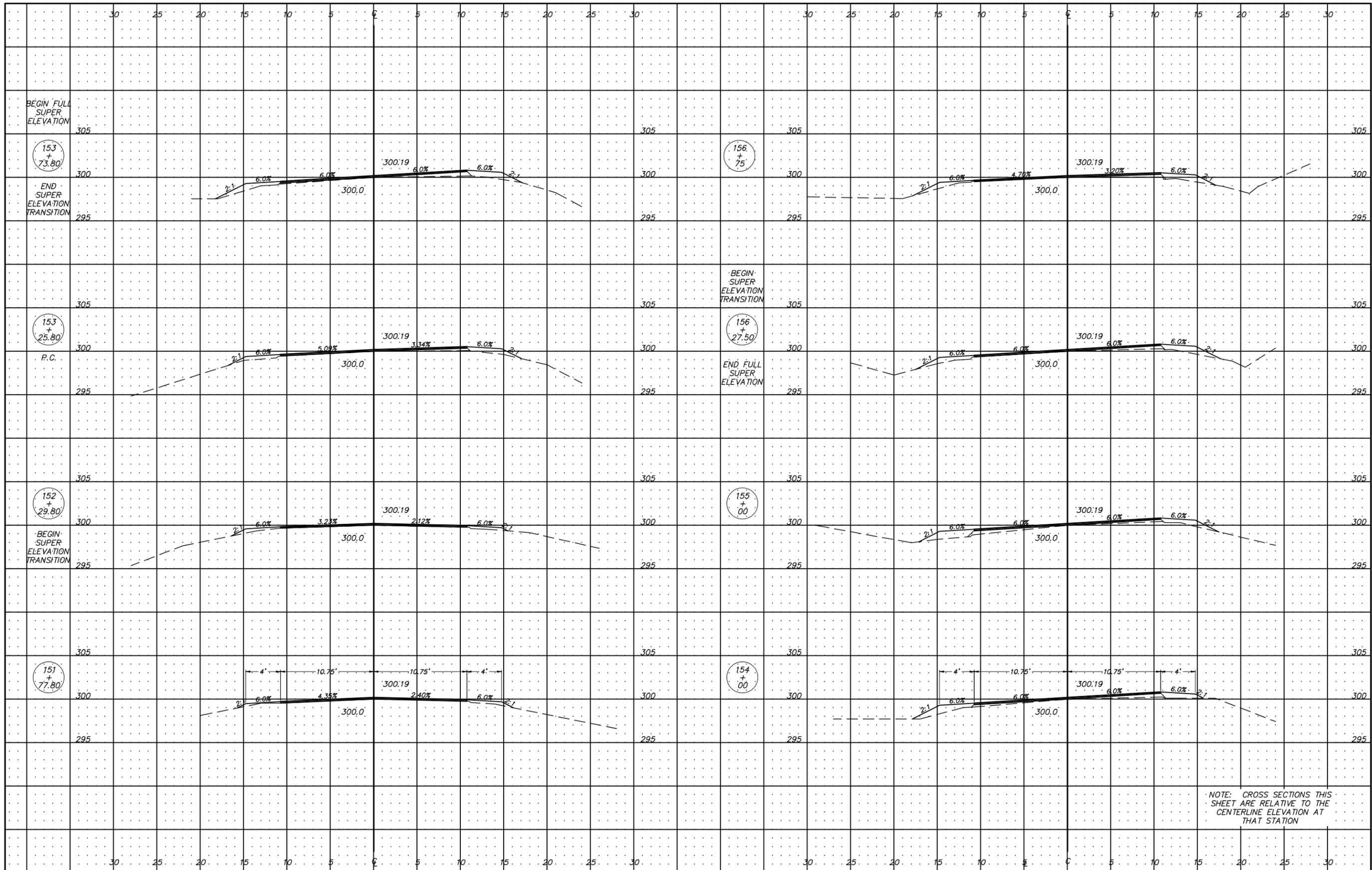
NOTE: CROSS SECTIONS THIS SHEET ARE RELATIVE TO THE CENTERLINE ELEVATION AT THAT STATION
