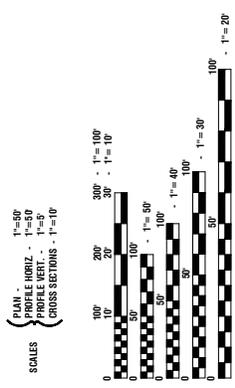
FULL SIZE PLANS HAVE BEEN PREPARED USING STANDARD ENGINEERING SCALES. REDUCED SIZED PLANS WILL NOT CONFORM TO STANDARD SCALES. IN MAKING MEASUREMENTS ON REDUCED PLANS, THE ABOVE SCALES MAY BE USED.
