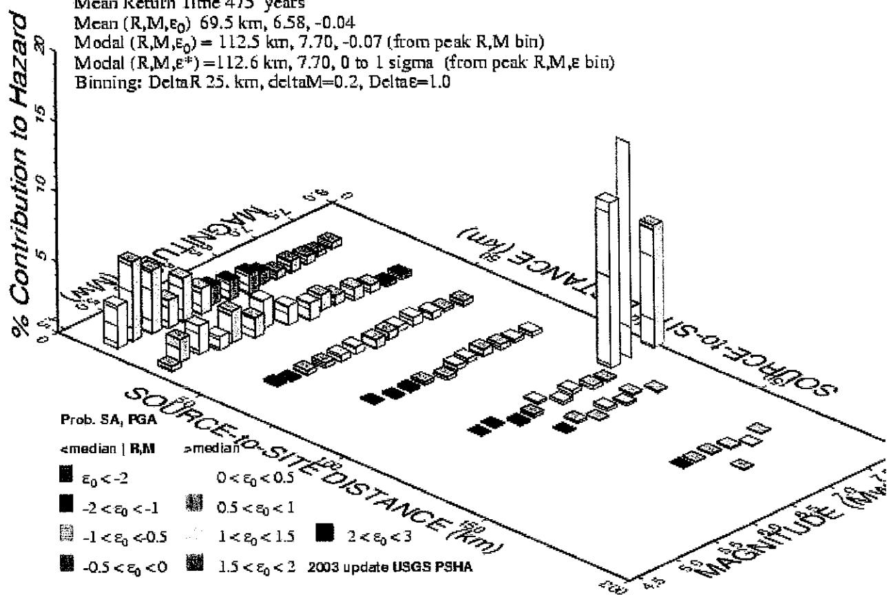
GMT 2009 Dec 10 19:10:14 Distance (R), magnitude (M), spallion (E,D,E) deaggregation for a site on ROCK avg Vs=760 m/s top 30 m USGS CGHT PSHA2002v3 UP DATE Bins with H 0.05% conf
