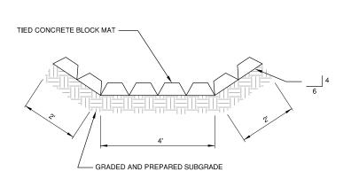
TIED CONCRETE BLOCK MAT SECTION C-C
