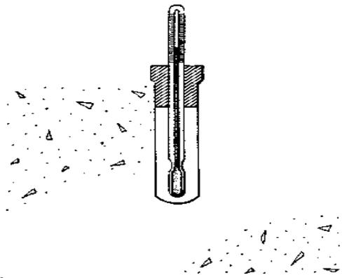
5. The exact method for surface and sub-surface concrete temperature monitoring shall be indicated in the contractor's cold weather concreting plan. The maximum permissible difference between the interior and surface temperature is 35 °F. Adjustments in protection method shall be implemented if the maximum permissible difference is exceeded.
